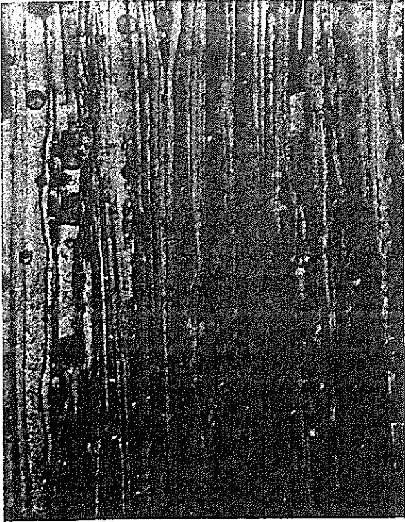
Figure 1.—Latewood tangential section from sapwood charge 63 Sontek. Note air bubbles distributed throughout the creosote in tracheids. 100 X.
